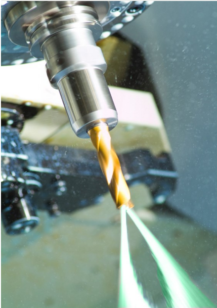
Hi-pressure through-tool machining with GreenCut Cutting Fluid.
